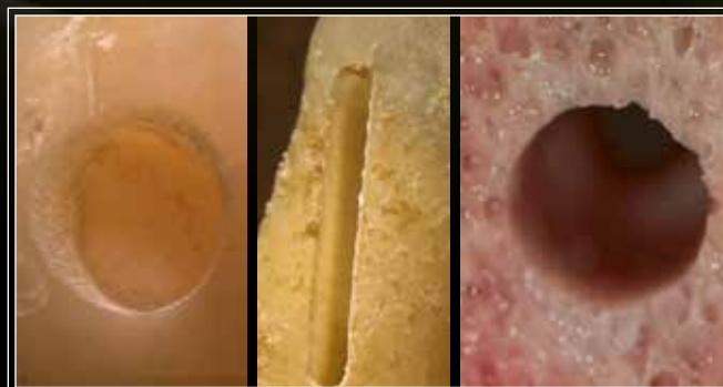
Samples of easily achievable scanning patterns in hard tissue drilling and cutting.
